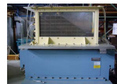
Shaking table test of slope under rainfall & earthquake
